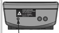
The laser beam exits the remote control through the smaller (left) opening on the front.
