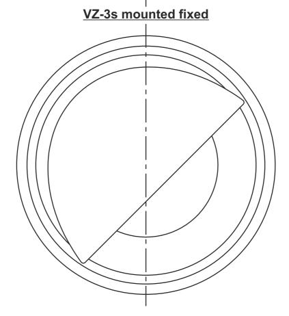
Turn swivel **top** plate counter-clock-wise to the end position.
