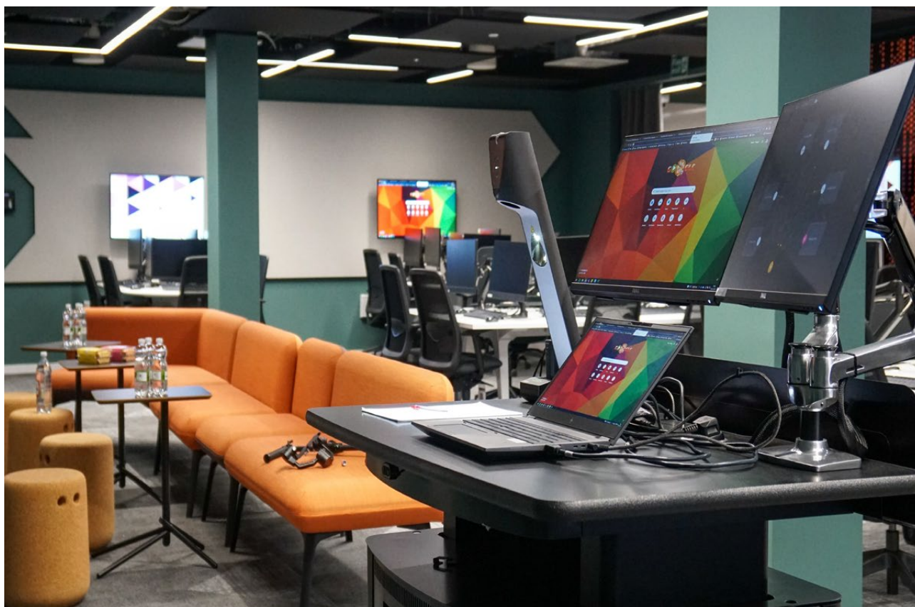
The lecturer's lectern with WolfVision Visualizer for display of physical content materials, plus a touch panel on the right with customised 'Room View' for control of the vSolution MATRIX system.
