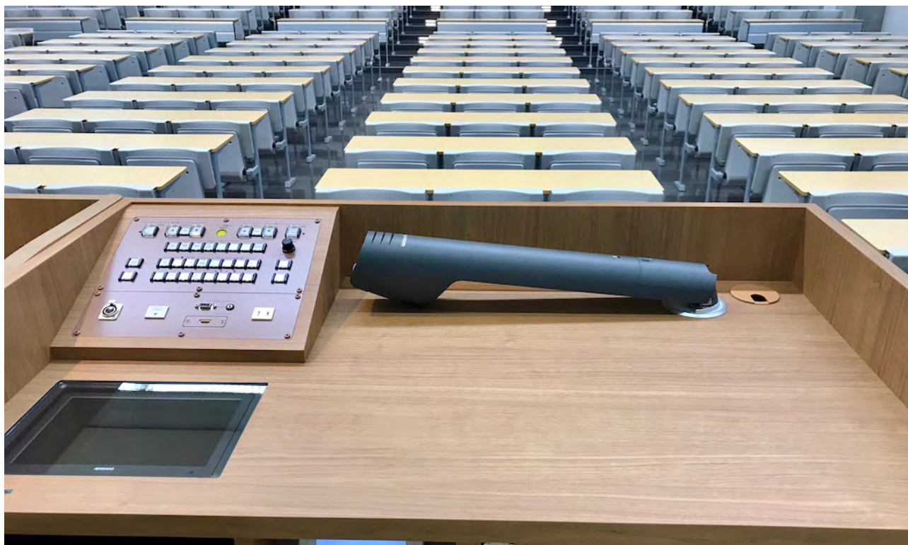
VZ-3neo Visualizer configured to fold down 90° to the left-hand side for space-saving convenient storage at Tokyo Keizai University.
