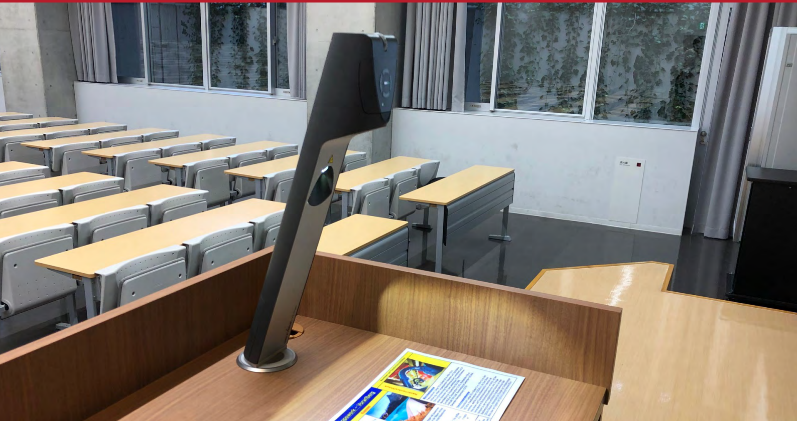
Tokyo Keizai University, Japan: VZ-3neo installed without working plate, directly onto a classroom lectern.
