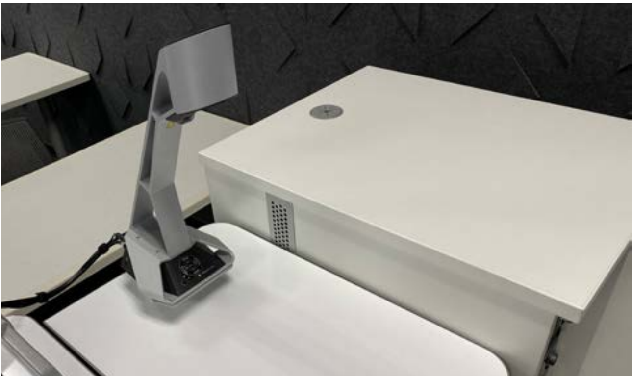
vSolution Cam installed on the optional Riser Plate in some classrooms to increase pick-up area, also showing laminated desktop pick-up area.
