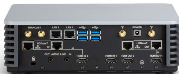
WolfVision Cynap with integrated HDBaseT modules.
